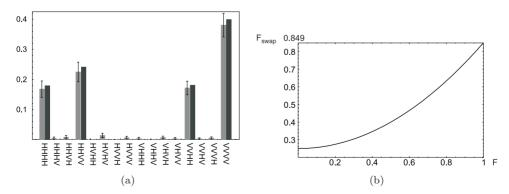
Fig. 3. (a) Measured (grey) and with  $\chi_{\rm mod}$  simulated (black) four photon detection probabilities for the cluster state  $|\mathcal{C}_4\rangle$ , (b) Calculated fidelity  $F_{\text{swap}}$  of the swapped states depending on the fidelity F of the two initial Bell pairs, using  $\chi_{\text{mod}}$  for the BSA.
