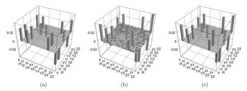
Fig. 2. (a)  $\chi$  matrix of the QPT for an ideal phase gate, (b) for the experimentally realized gate and (c) for a theoretical model fit to the experimental data. The imaginary part of the experimentally obtained  $\chi$  consists of noise only which is comparable to the one in the real part.
